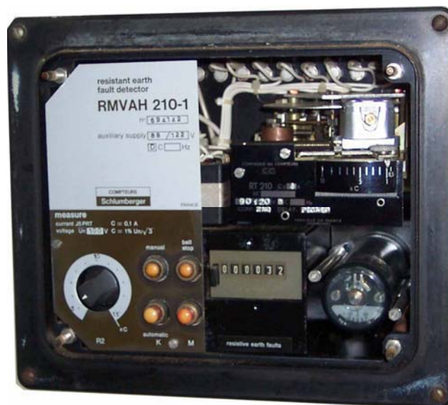
Gambar 3.30. Restristant earth fault detector
